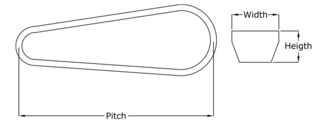
$\begin{array}{ll} \text{Datum Llength} = 5440 \\ \text{Height} &= 12 \\ \text{Length inside} &= 5405 \\ \text{Type} &= \text{CC210} \\ \text{Width} &= 22 \\ \end{array}$
